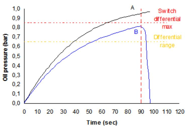
Figure 2-12 Oil pressure difference switch starting phase
