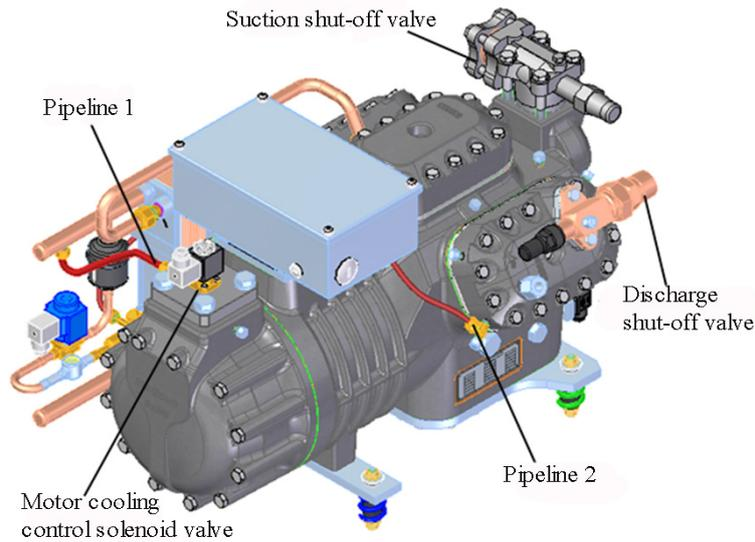
Figure 3-3 Pipeline diagram of expansion valve kit with liquid subcooler
