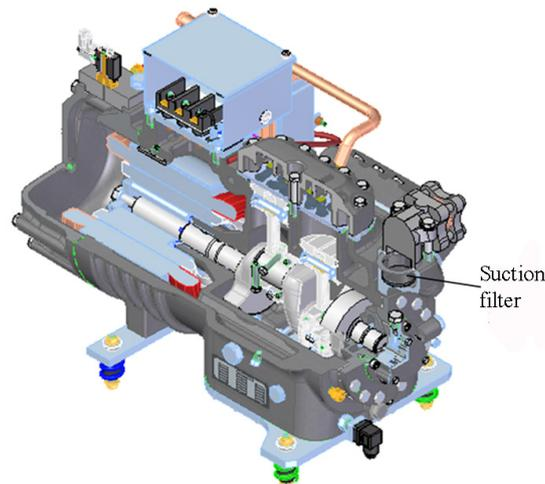
Figure 4-2 Position of the SB6C series suction filter
