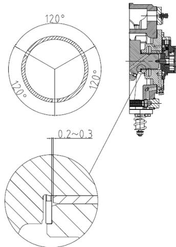
Figure 4-9 Schematic diagram of oil pump base bushing
