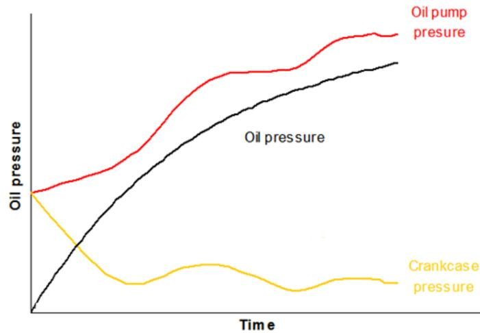
Figure 2-4 Oil pressure difference-time chart during compressor startup
