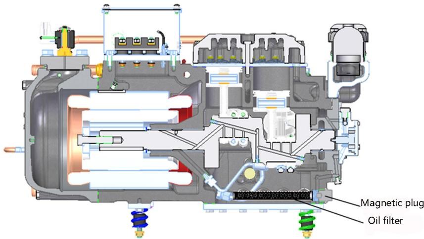
Figure 2-6 SBC series oil filter
