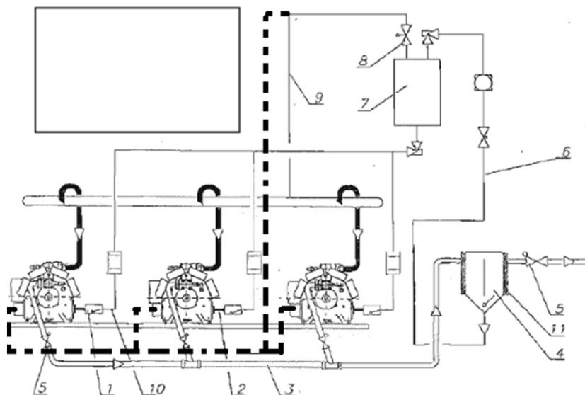
Figure 12-1 Parallel compounding with oil level regulators and single oil separator
