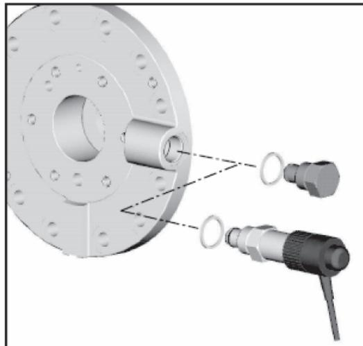
Figure 2-17 Installation diagram of the electronic oil pressure difference switch
