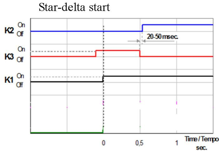
Figure 5-3 (b) Schematic diagram of the star-delta start contactor delay
