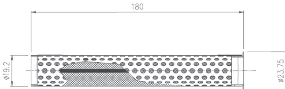
Figure 2-7 SBC series oil filter
