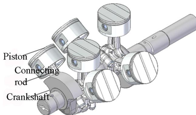
(b) Schematic diagram of the mutual position of the crankshaft, connecting rod and piston
