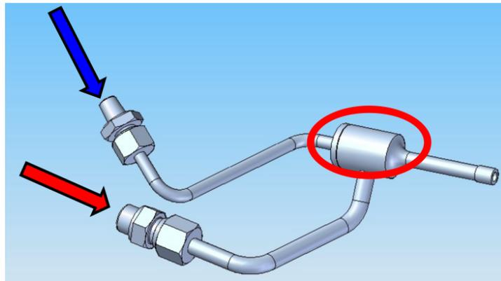
Figure 2-21 Oil return ejector
