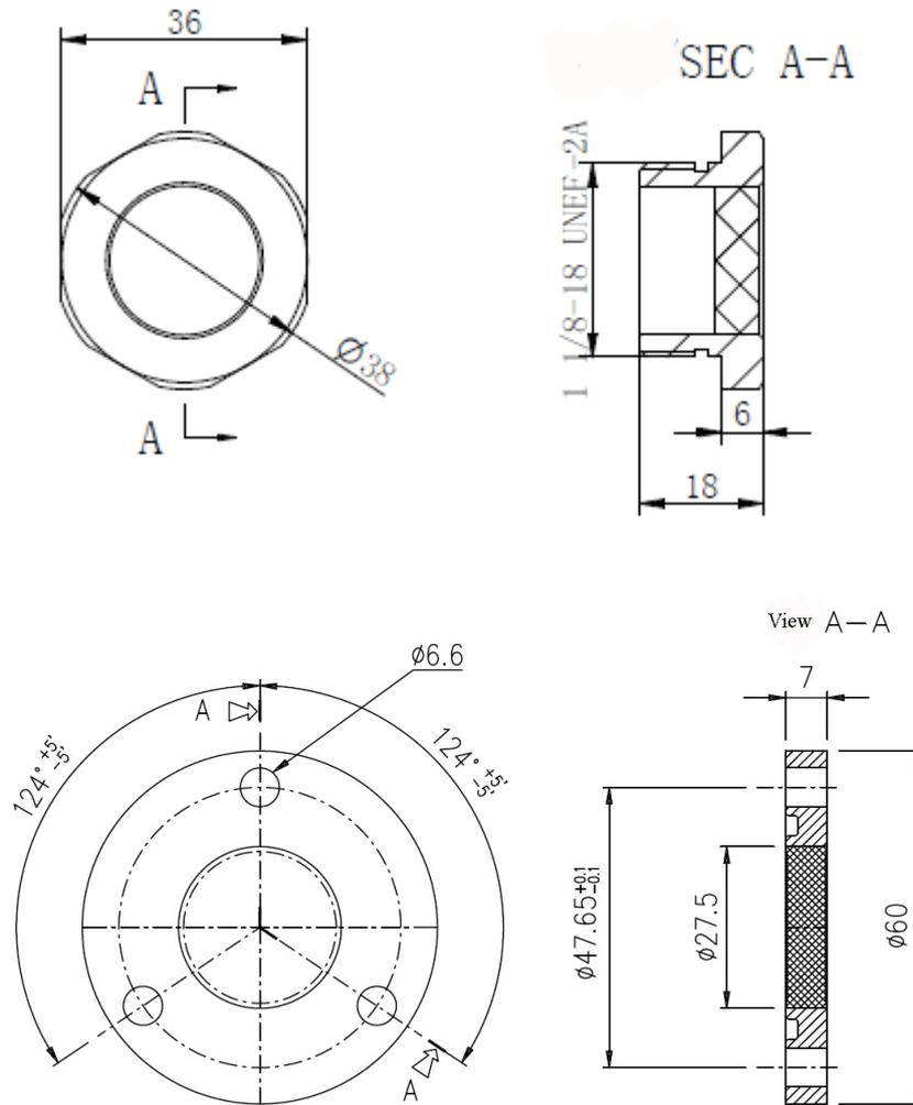
Figure 2-11 Overall dimension drawing of oil sight glass
