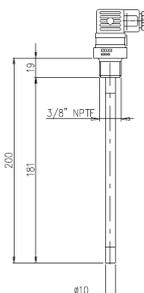
Figure 2-9 Crankcase heater overall dimension
