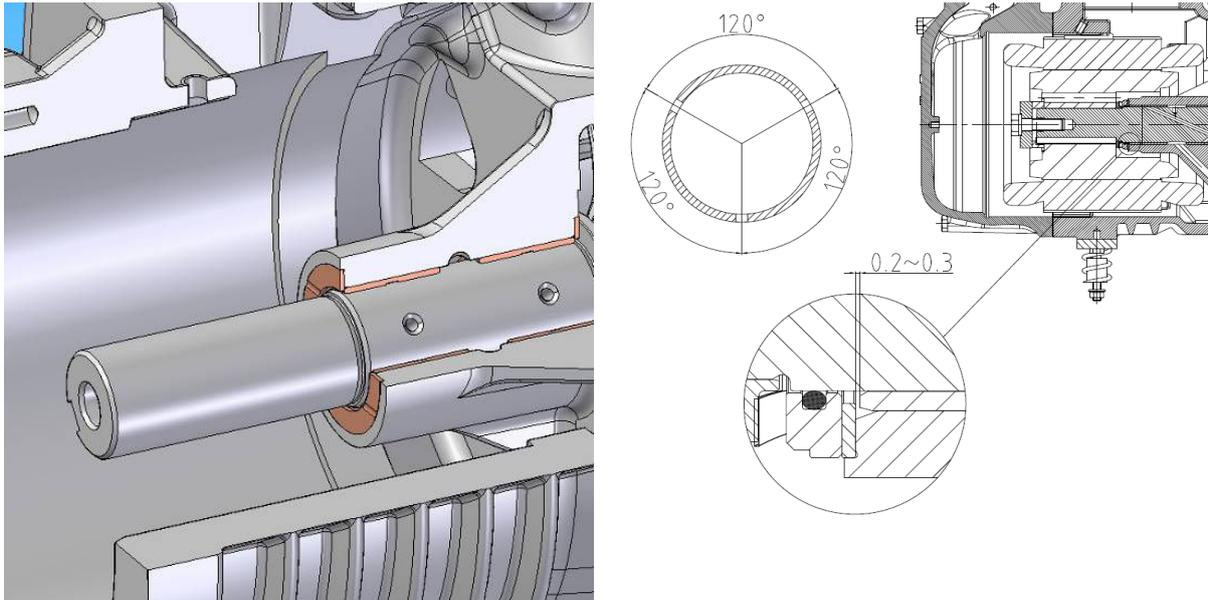
Figure 4-8 Schematic diagram of the motor side bushing
