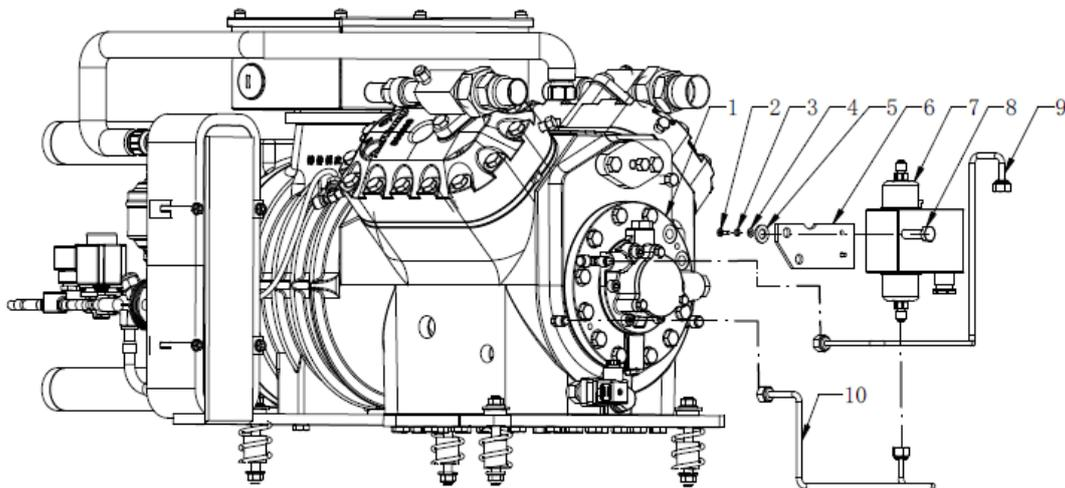
Figure 2-19 Mechanical oil pressure difference controller MP54 components (code: 303191)
