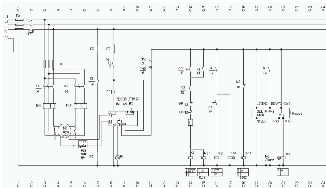
Figure 2-16 Electrical wiring diagram of electronic oil pressure difference switch
