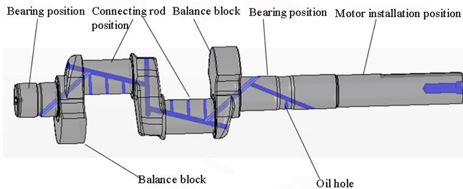
(a) Schematic diagram of SBC series crankshaft
