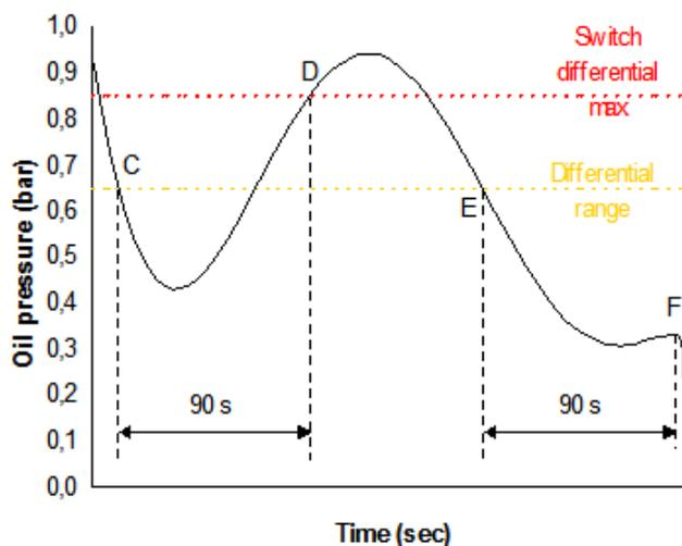
Figure 2-13 Oil pressure difference switch operation phase
