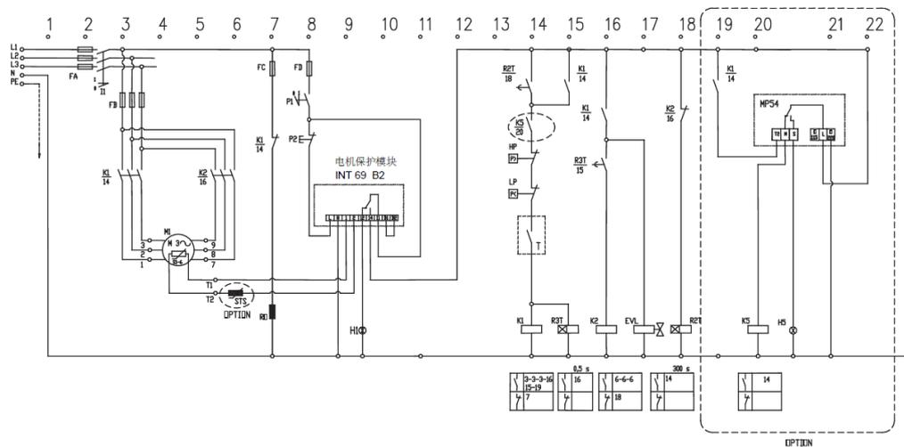
Figure 2-29 Electrical diagram of mechanical oil pressure difference switch MP54 application
