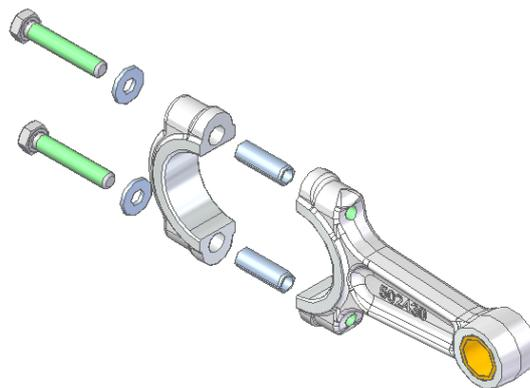
Figure 4-5 Schematic diagram of the SBC series connecting rod components
