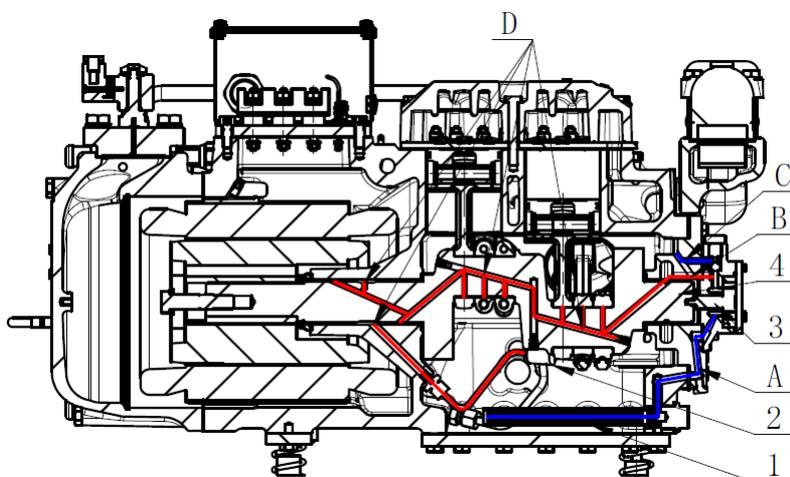
(b) Schematic diagram of SBC series forced lubrication
