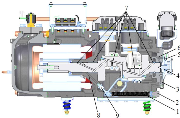
(a) Sectional view of SBC series compressors forced lubrication
