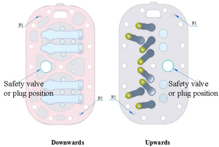
(a) Schematic diagram of the first stage compression valve plate
