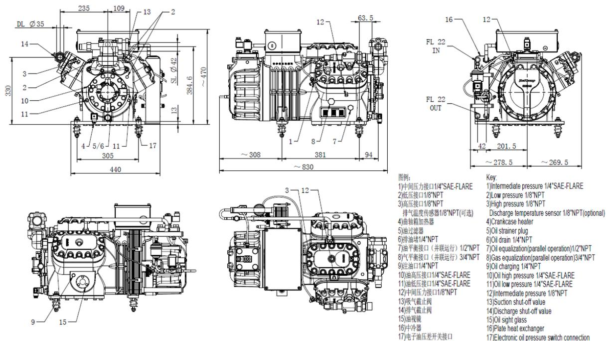
Figure 8-2 Overall dimensions of model SB6C-1600 ~ 3000
