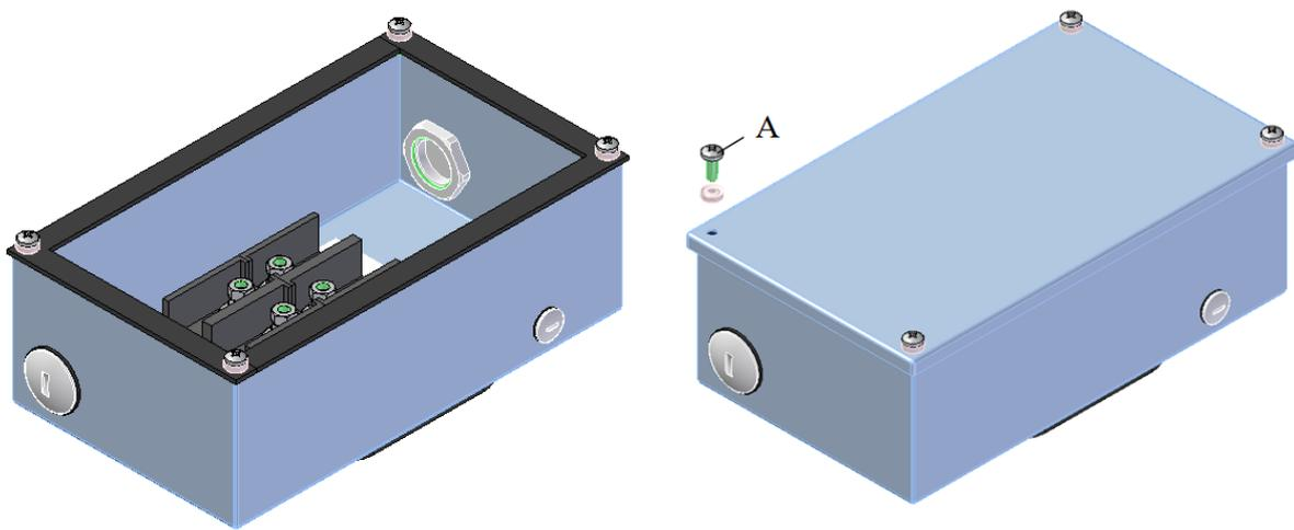
Figure 5-5 Schematic diagram of terminal box
