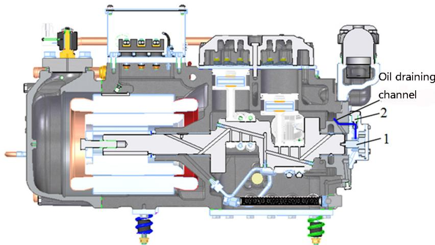
Figure 2-3 SBC series oil safety valveNotes
