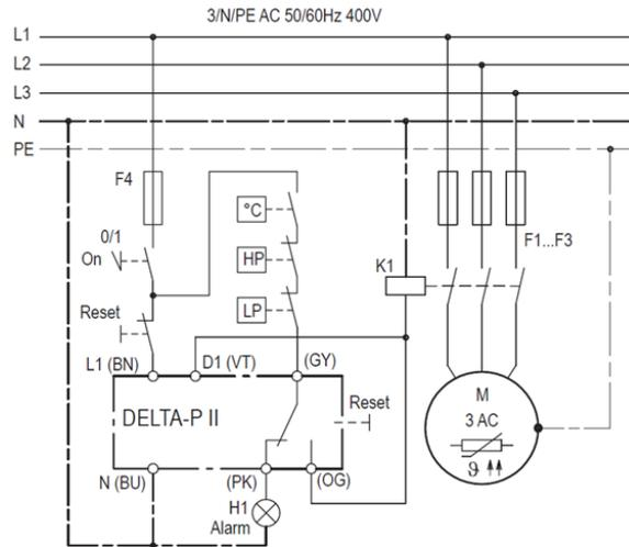
Figure 2-15 Wiring diagram of electronic oil differential pressure switch
