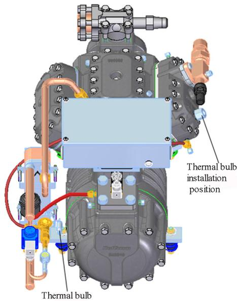
Figure 3-2 Expansion valve kit with liquid subcooler
