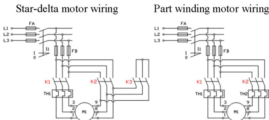
Figure 5-3 (a) Wiring diagram of the star-delta motor and part winding motor
