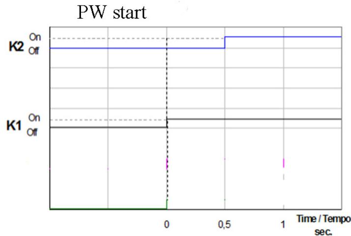
Figure 5-3 (c) Schematic diagram of the part winding start contactor delay
