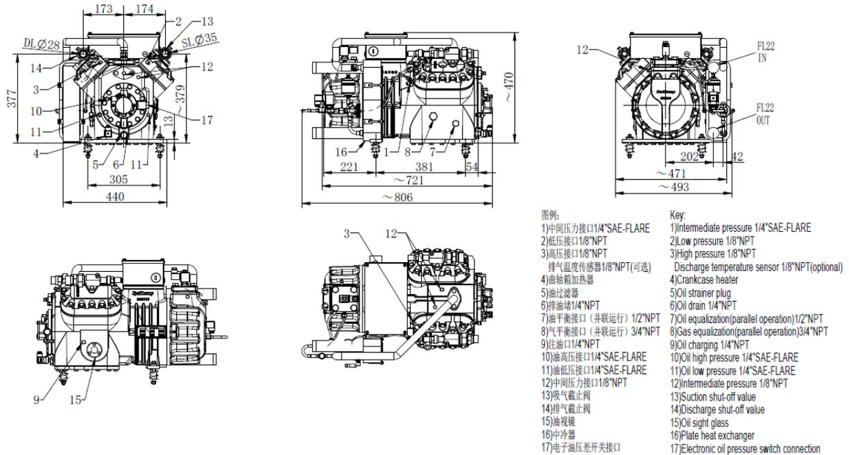
Figure 8-1 Overall dimensions of model SB4C-1200/1400
