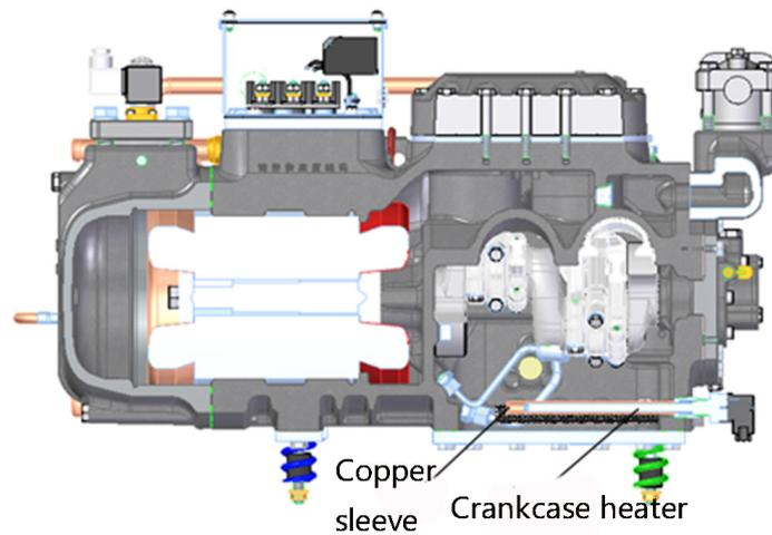
Figure 2-8 SBC series crankcase heater
