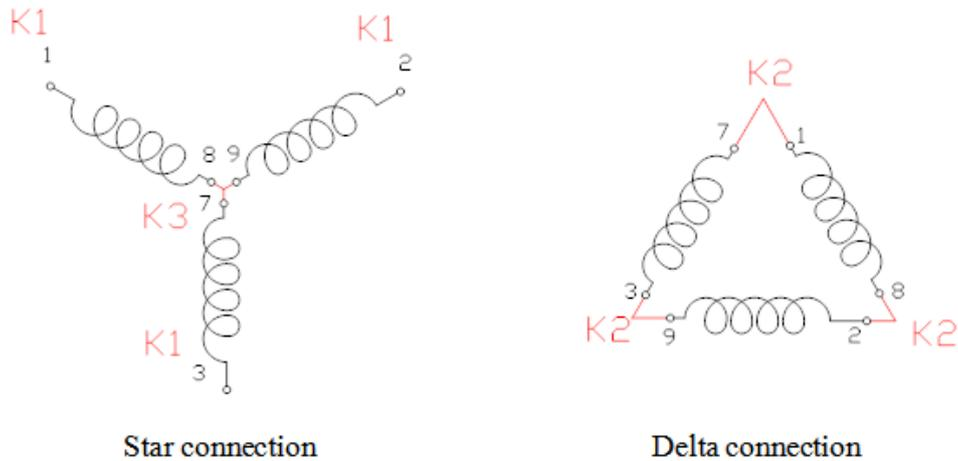
Figure 5-2 Connection diagram of star-delta
