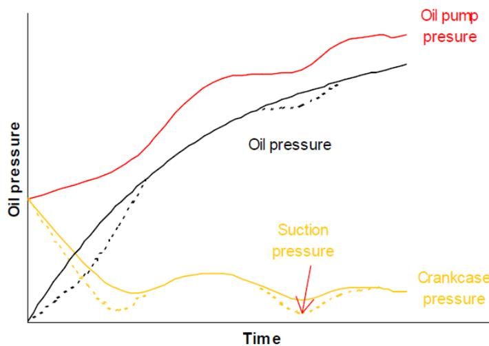
Figure 2-5 The oil pressure difference-time curve between the suction part and the crankcase equipped with check valve
