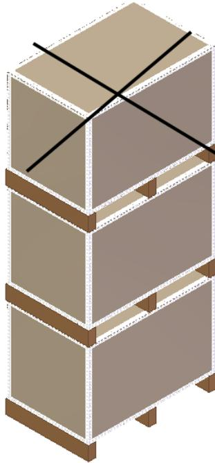
*Figure 8-5 Two layers are the Max. layer*
