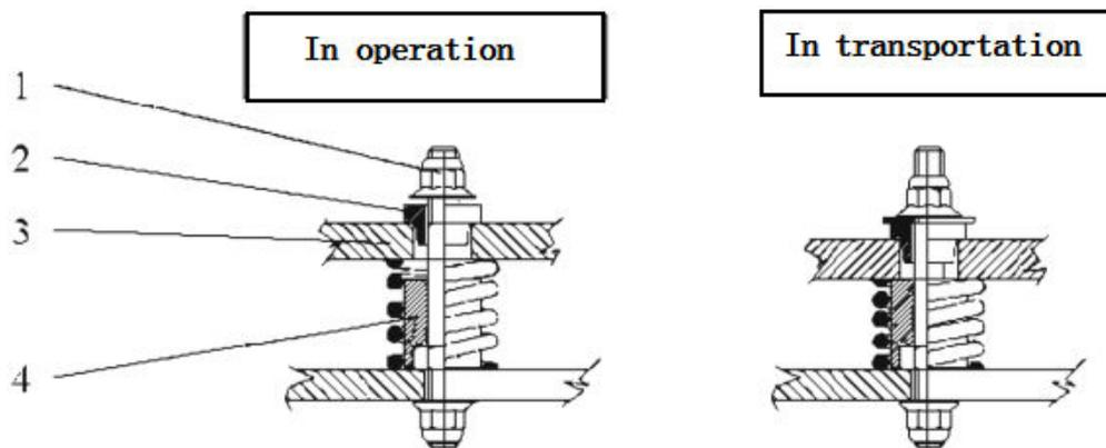
Figure 8-8 The different shapes of spring pad during operation and shipment of the compressor
