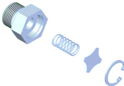
Figure 2-23 Explosion drawing of anti-foaming check valve
