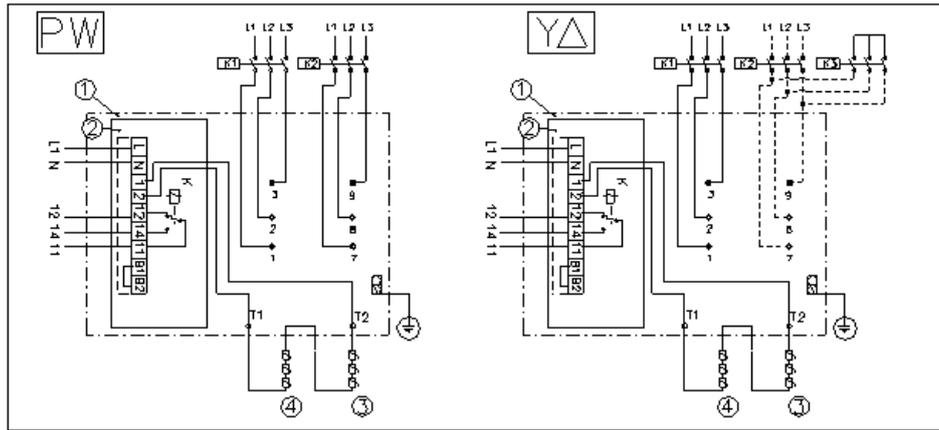
Figure 5-4 INT69 B2 electrical wiring diagram (PW wiring and star-delta wiring)
