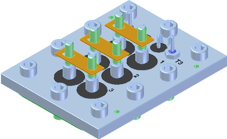
Figure 5-6 DOL connection diagram
