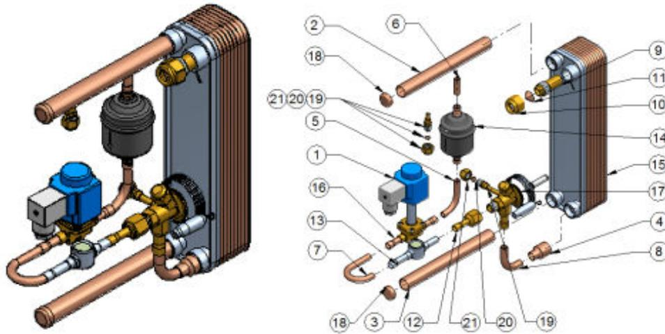
Figure 3-1 Explosion diagram of expansion valve kit with liquid subcooler
