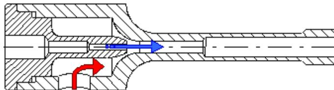
Figure 2-22 Venturi ejector profile view
